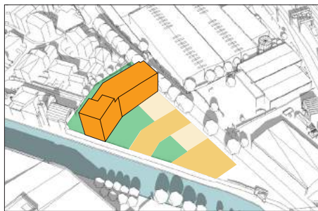
5 Establish northern boundary with low-rise massing which meets sunlight and daylight criteria
